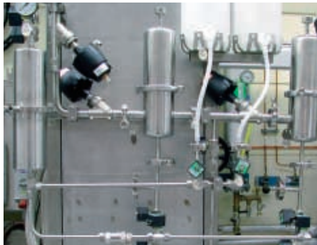
Optional dual sterile membrane filters arranged in series with optional in-place automatic WIT integrity testing.
