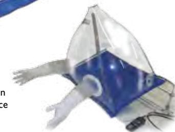
Optimal air-tightness of the enclosure (Factory tested: compressed air inflation at 2.5 mm Hg, a certificate of compliance is provided with each enclosure)
