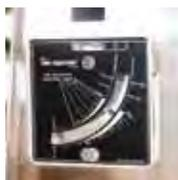
This system continuously monitors the face velocity, which must fall between 0.4 and 0.6 m/s. (in accordance with the requirements of the AFNOR NF X 15-211: 2009 standard).
