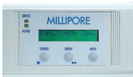
Automatic Sanitization Module control panel
