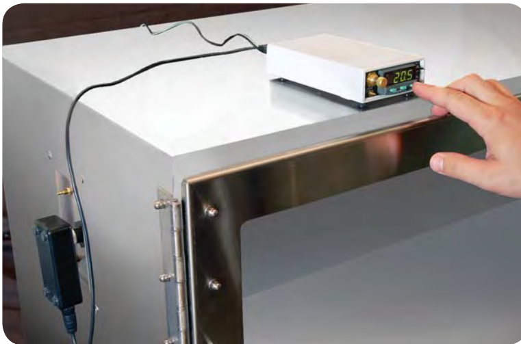
The ProOx P110 integrates with A-Chambers via stainless steel adapter plate.
