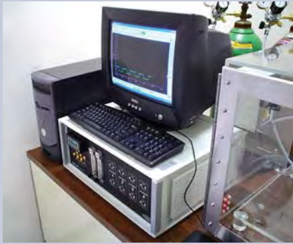
The OxyCycler A44C can use a PC interface (desktop or laptop) to control and monitor carbon dioxide with ease.
