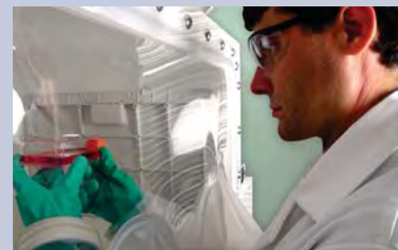
Soft comfortable glove front makes sealed barrier between inside and outside. Less contamination risk than standard open BSL hood.
