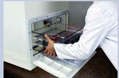
Cells can be safely moved in and out of Xvivo System inside transport chambers and subchambers without exposure to room contaminants or disturbances to O 2 and CO 2 .
