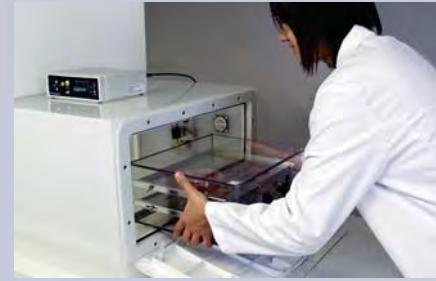
Cells can safely be moved into and out of I-Glove inside subchambers and transport chambers without disturbance to O 2 and CO 2 , or exposure to microbes in lab.
