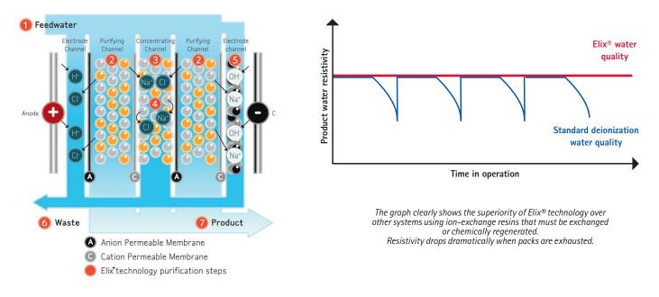
EMD Millipore's Elix® module: unique technology based on anion-permeable and cation-permeable membranes; high-quality ion-exchange resin; and activated carbon beads.
