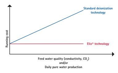
Running costs for a water purification system using Elix® electrodeionization technology or standard ion-exchange resins that must be exchanged or chemically regenerated: With Elix® technology, running costs remain constant, and are independent of feed water quality or pure water use.
