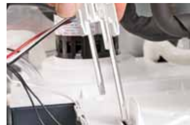
Electric conductivity-based water sensor
