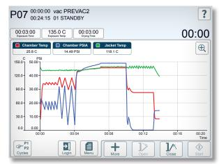
**Plot Graph:** Displays cycle temperature and pressure in a color graph plotted over time
