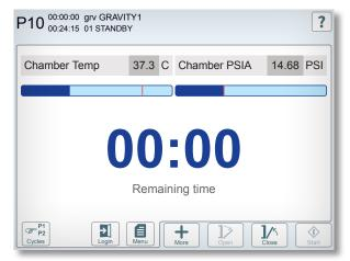
**Bar Graph:** Displays temperature and pressure in a bar graph with large, easy-to-read time remaining in the center
