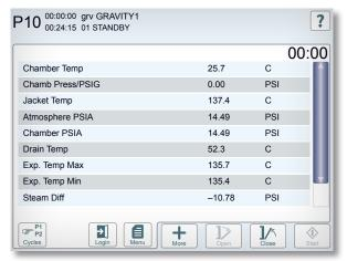
**Detail Display:** Displays real time process information in text form
