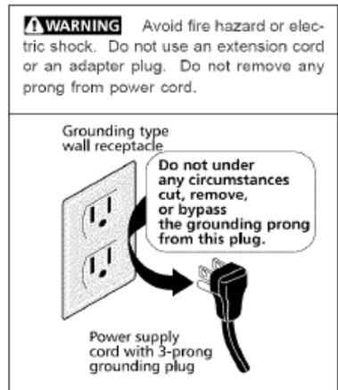
Be sure your unit is properly grounded. Use the 3-prong plug provided into a 3-prong grounded outlet. Unless the above grounding method is followed, you are not protected against severe or lethal shock in the event of a short circuit of an electrical component or wiring of the unit.
