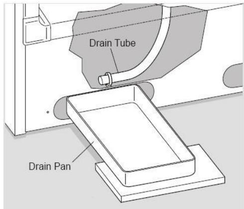
drain out. Check the pan occasionally to ensure it does not overflow. A ½ inch garden hose adaptor (available at most hardware stores) can be used to drain the freezer directly into a floor drain. Replace the drain plug when defrosting is complete so warm air does not enter the freezer through the hole.
