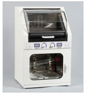
HM-4000 Multidizer Two compartments operate independently with shake, rock, roll and rotate motions
