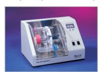
HB-500 Minidizer Compact and portable, this unit is designed for low throughput use.
