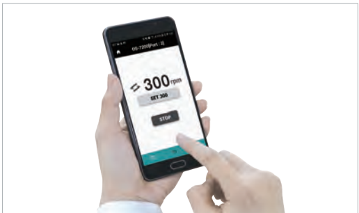
Mobile monitoring and control via mobile application. (Option)
