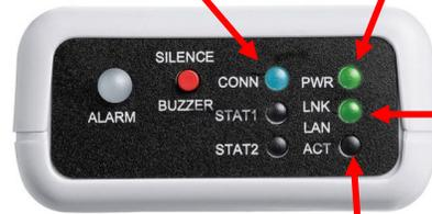
**LAN LNK:** Solid green when the LAN hardware connection is good
