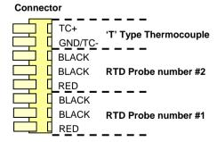
**NOTE:** for RTD probes that have 2 red and 1 white wire, connect the white wire to the terminal marked RED and connect the 2 white wires to the terminals marked BLACK.
