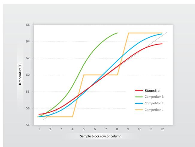
The Linear Gradient Tool (**LGT**) enables programming of a temperature gradient with defined temperature intervals (increment) between the individual rows of the sample block. It allows the user to enter the calculated  $T_m$  value minus, e.g., 5 °C and the desired temperature increment (e.g.  $\pm 1$  °C) between the rows of the sample block. For maximum comfort, the Linear Gradient Tool now supports programming of even-numbered temperature values for a maximum number of rows.
