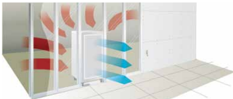
Positive / Negative Room Pressure Application
