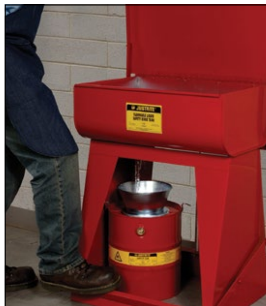
Position drain cans under rinse tanks to safely collect used solvents.
