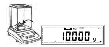
9. Once an accurate count has been taken, the container and its contents may be removed from the scale.
