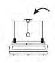
10. The weight of the plunger will be displayed. Once the weight is stable, press the P key. Command "M1" will be displayed, indicating that the weight of the plunger has been stored in the formula.
