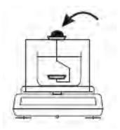
10. Once the weight of the object stabilizes, press the P key. Command "M1" will be displayed indicating that the weight of the object in air has been stored in the formula.
