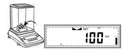
8. Once an accurate count has been taken, the container and its contents may be removed from the scale.
