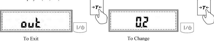
6. After the T key is pressed, in order to set a new AZSM range a dash will be displayed indicating a new AZSM value between 0.1d and 5d should be entered.
