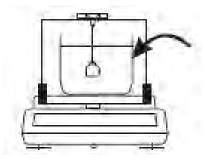
12. As the plunger displaces the liquid in which it is submerged, the weight will decrease. Once the new weight stabilizes, press the P key.
