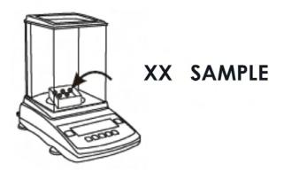
3. The weight of the sample will be displayed as it is placed on the pan. Once the weight of the sample stabilizes and the stability indicator appears on the display, press the MENU key to enter the main menu.
