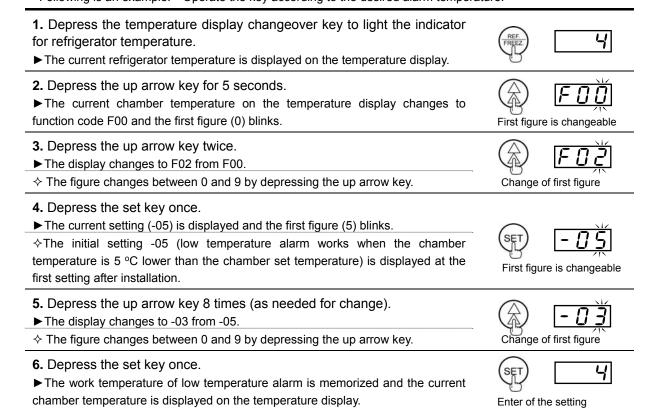
♦ The setting mode returns to the temperature display mode automatically when 90 seconds has passed without any key operation (auto-return function). In this case, the setting is not accepted.
