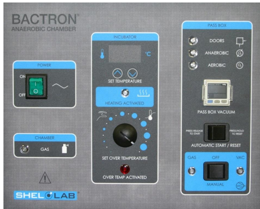
Figure 23: Main Control Panel
