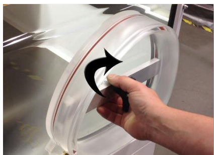
Figure 22: Installing / Closing the Arm Port Doors
