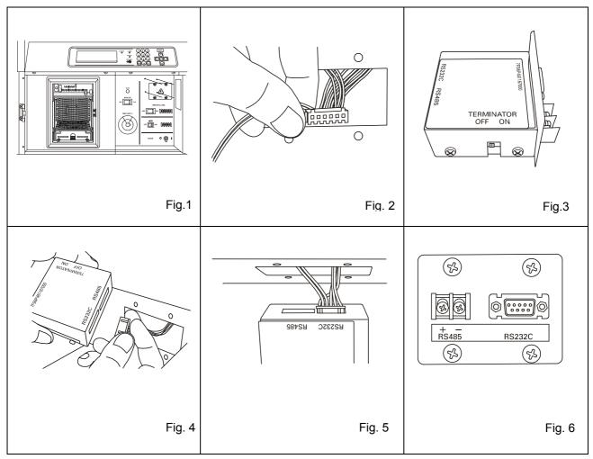
\* When a data transmitting function to the personal computer is done, an interface board MTR-480 (option goods) and communication cable of 9 pin Dsub cross type for RS232C are necessary.
