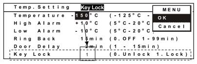
**2.** The cursor is moved to the password column (Password). Input 4-digit password and press the enter key (ENTER). The buzzer sounds shortly and the key lock is released. The "Key Lock" indication of the temperature setting screen (Temp. Setting) disappears.
