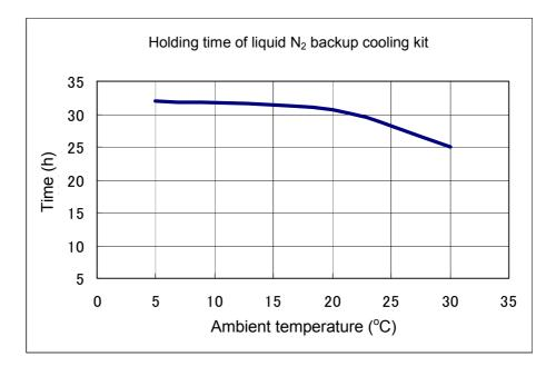
• The above data is the experiment value which uses liquid N<sub>2</sub> 100L. (no-load)
