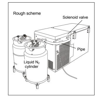
**6.** This completes the setting of the tank for automatic spouting in case the freezer temperature should match the alarm set temperature.
