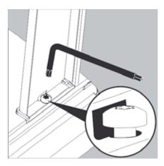
6) Turn the key approx. two times to loosen the Torx screws.
