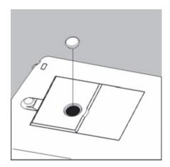
Lift cover plate out of the bottom of the balance.
