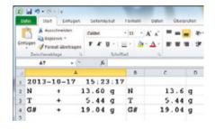
▶ With the "PC spreadsheet format" setting on the balance, Microsoft Excel 2010 has the following display for the "Gross/ Tare/Net" example
