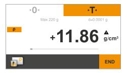
▶ The balance calculates the density of the sample and displays this value.
