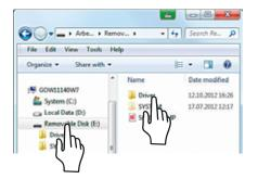
➤ To install the installation program for the USB driver on the PC: Click on the appropriate removable data carrier (in this case, the E: drive) and then click on the **Driver** folder.
