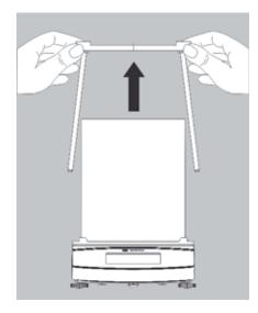
and remove the draft shield frame by pulling up.
