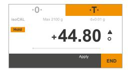
➤ The maximum measured weight value is displayed and kept as long as the sample remains on the balance.
