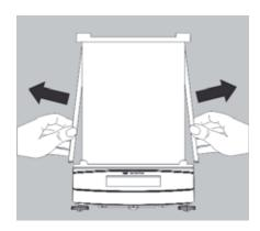
7) Pull out the draft shield frame from the side of the guide
