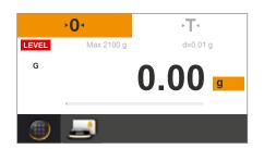
▶ When LEVEL appears in red at the top left of the display, you must level the balance.
