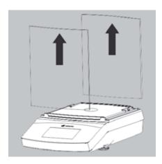
8) Pull out the front and rear glass panels (upwards).
