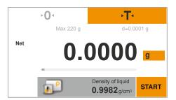
▶ The balance is tared with the prepared density determination kit.
