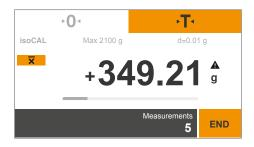
➤ The specified number of measurements is carried out. The average is calculated and displayed.
