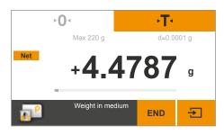
ightharpoonup The weighing display shows the step **Weight in medium**.
