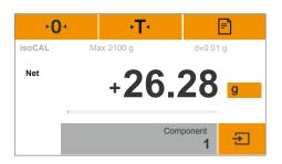
> If a printer is connected, an additional button automatically appears at the top right of the display.
