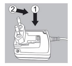
Push (1) and slide (2) the power plug adaptor (A) required for the power supply into the opening of the AC adaptor module (B). When doing this, the AC adaptor needs to lock into position.
