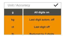
The left list contains the available units. The currently selected unit is marked (e.g., **g**). The most recently selected units automatically appear at the top of the list. Units which are rarely or never used are shown further down the list. The right list contains the display accuracy options. The currently selected setting is marked (e.g., **All digits on**).
