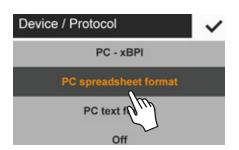
To access the **PC spreadsheet format** menu option on the balance: Go to **USB port** and select the **Device / Protocol** option.
