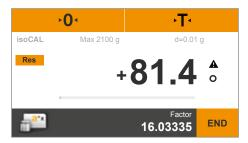
➤ The weight of the sample is multiplied by the entered factor, and the result is displayed.
