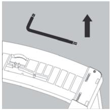
▶ Remove the Torx key up from the draft shield under the cover.
