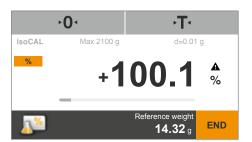
➤ The balance shows the percentage of the sample based on the reference sample.
