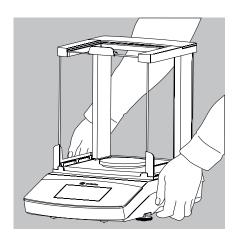
► Hold the balance under the housing, lift it up carefully, and carry it to its new location.
