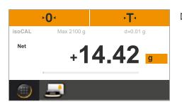
> The measured value can be read as soon as the weight value stops changing and the unit is displayed.
