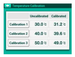
Touch the temperature on Set Temp. and put the desired temperature on it and operate the unit. Wait until the actual temp reaches to the setting temp. Once the actual temp reaches to the setting temp, touch the calibrated temp and put the temperature from the external sensor. Touch the confirm for the saving. The unit stops the operating. The unit read the temp as the external sensor's value.
