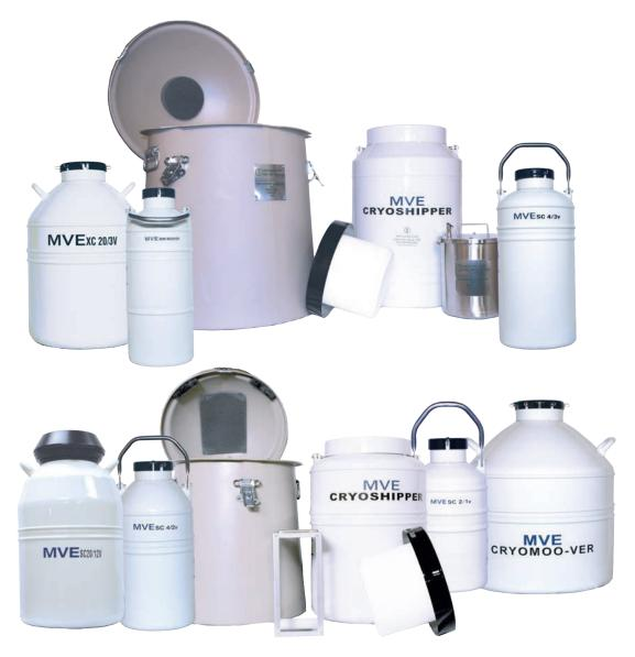
MVE Vapor Shippers are designed for the safe transportation of biological samples at cryogenic (-150°C or colder) temperatures. Manufactured from durable, lightweight aluminum, the MVE CryoShipper Vapor Series employs a hydrophobic compound which absorbs the liquid nitrogen to ensure dry, spill-free vapor-phase shipping.
