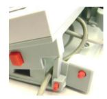
Thread printer cable along cable coils on bottom of balance. Or pass cable through groove near release button.
