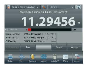
Once the necessary weights have been determined, the density of the sample is displayed in **g/cm**<sup>3</sup> (along with the weight in air, un-oiled and oiled, and weight in water) on the Application screen
