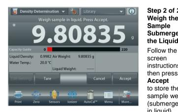
Step 2 of 2 -Weigh the Sample Submerged in the Liquid.
