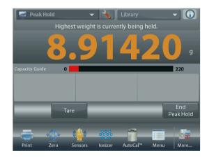
Clear the pan or press **Tare** to reset the display and re-start the process.
