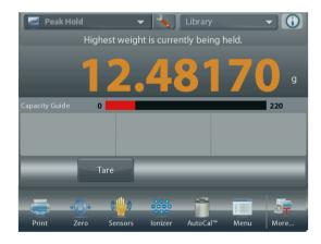
The highest stable weight reading is held until the weight is removed.
