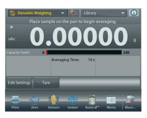
Place specimen on the Pan. The cycle starts automatically.
