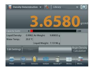
Once the necessary weights have been determined, the density of the sample is displayed in g/cm<sup>3</sup> (along with the weight in air, weight in water) on the Application screen.
