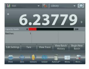
To view the Process results graphically (batch comparison), press the **View Trace** button.
