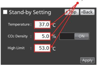
**2.** Press Numerical key or Up/Down key to input numerical value, and press OK key.
