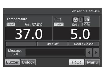
2. CO<sub>2</sub> gas supply line A is changed to B.
