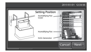
**13.** On the  $H_2O_2$  Decontamination Step1 screen, the system check starts automatically. If the system is normal, the display leads the  $H_2O_2$  Decontamination Step2 screen. When the system is abnormal, refer to Table 8 on page 82.
