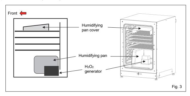
**10.** Make sure that the duct, the fan and the  $H_2O_2$  generator are securely attached (refer to Fig. 1 to 3 on page 85). After that, close the inner door and the outer door.
