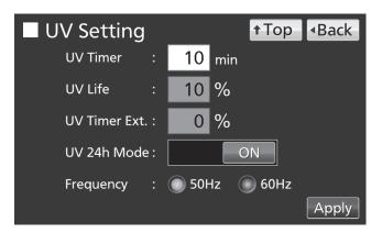
**8.** The UV lamp lights continuously for 24 hours. "UV : ON" is displayed on the UV lamp condition display when UV lamp is lighting.
