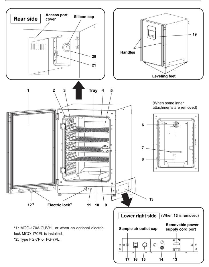
**1. Outer door:** The outer door is held to the frame with the magnetic seal. The door heater is installed in the door panel. The door opening is reversible. Contact our sales representative or agent to change the door hinge from left to right or vice versa.
