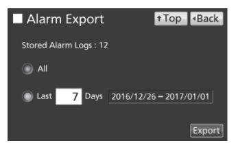
**7.** Even after completion the export of alarm log data, Information dialog box is displayed. Press OK key.
