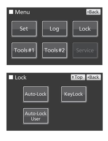
4. Press KeyLock key to display the Key Lock
