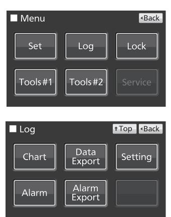
**4.** On the Setting screen, input Log Interval. Press Apply key to save the input value. The display returns to the Log screen. Settable range: 2 minutes~30 minutes.
