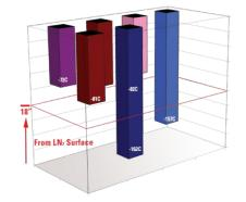
Liquid Nitrogen Freezer, Uniformity Gradient Potential (vapor phase)
