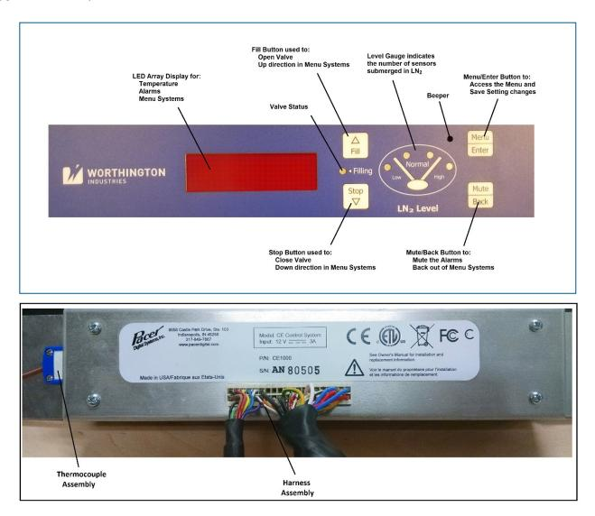
Connect the thermocouple plug of the harness assembly into the control at the thermocouple plug. This is located on the right edge of the control if looking at it from the front. One of the blades on the plug is slightly wider insuring that it is plugged in correctly. Copper blade should plug into copper colored plug. On the other end of the harness, connect the Thermocouple assembly into the plug insuring that copper colored blade is plugged into copper colored contact on receptacle.
