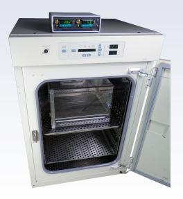
C-Chamber sits inside your incubator, and is connected to the controller which sits outside the incubator. C-Chamber can be removed from incubator and transported to remote locations without risk of disruption or contamination of cells inside.
