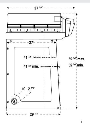
Heights according to the filtration column configuration
