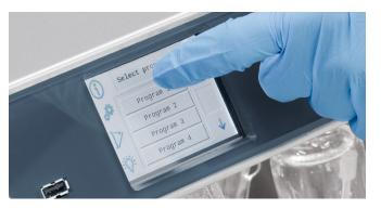
The Prolux PLC Controller includes a touchscreen interface with a common icon directory that permits scrolling access to primary screens from the same menu. A set of sub-menu screens display additional icon directories specific to the screen functions.
