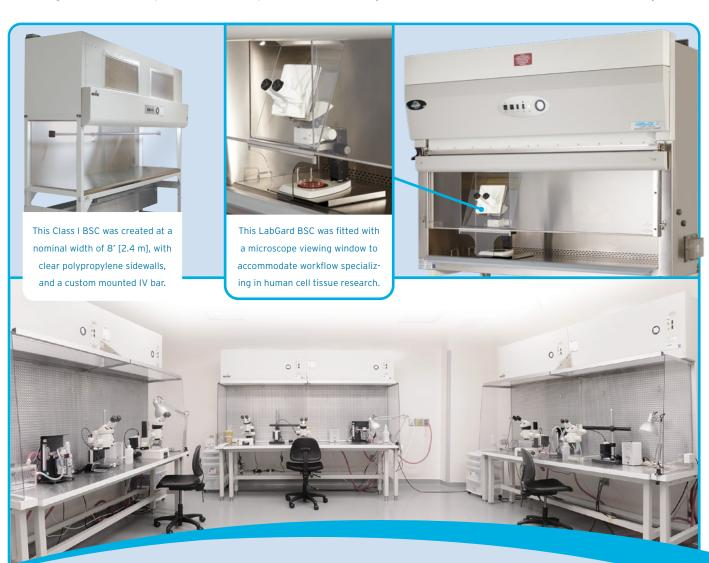
A custom model NU-240 was designed to offer a broader and taller work zone to accommodate a single workflow process involving microscopes. A customized isolation table was added to eliminate vibration in the work surface. The extended work surface allows a technician to perform several protocols without having to leave the work zone.
