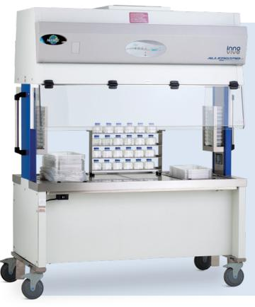
The AllerGard NU-620M is designed specifically to accommodate Innovive® disposable mouse cages while employing similar airflow mechanics as our other dual-sided models, by flushing the work zone with a vertical "piston of air" to preserve aseptic conditions.
