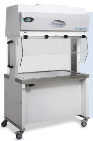
The AllerGard™ NU-621 Single-Sided Animal Transfer Station offers improved allergen protection by creating a dynamic air barrier of 75 fpm (0.38 m/s) at the front of the workstation. The HEPA filtered laminar downflow air of 60 fpm (0.30 m/s) maintains aseptic conditions within the work zone.
