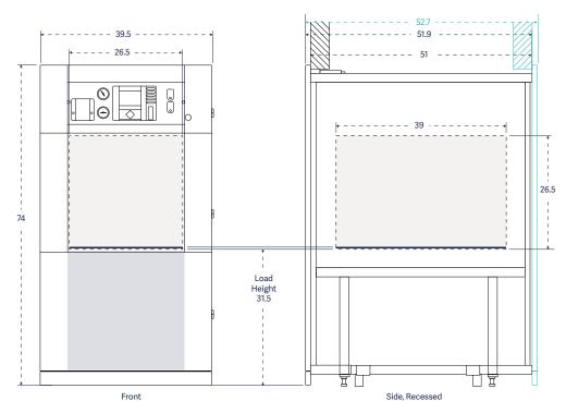
Side view illustrates facility wall cross section. Cabinet depth permits one-wall or two-wall recess. Requires wall opening cut-out size of 38"W × 73.25"H (965 × 1861 mm) prior to installation.
