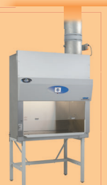
Type B1 30% Recirculated / 70% Exhausted Hard Connection External Vent
