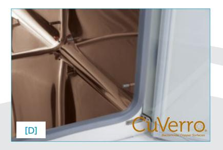
The best method to reduce the probability of contamination is to clean the interior of the incubator often, this includes all nooks and crannies (shelves, brackets, etc.) and to change the water pan (if using) routinely.
