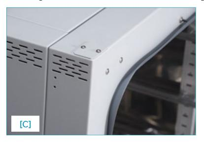
the seal around the inner door. The gasket is an area where humidity can build resulting in the growth of contamination if left unchecked. Make sure the gasket is removable and easy to clean. If using a v-gasket beware of the direction of the flap. A flap that points outwards towards laboratory [C] will collect particles keeping from entering the growth chamber. A flap that points inwards in an area for humidity to collect breading ground for contamination.
