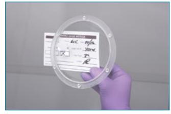
A magnifying glass in installed in the window sash enhances text written Exterior stainless steel shelf for collection of dirty mouse or rat cages. on animal identification cage cards.
