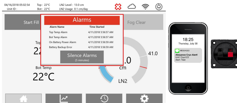
Alarm Notifications: local audio/visual, remote text and email, dry alarm contacts
