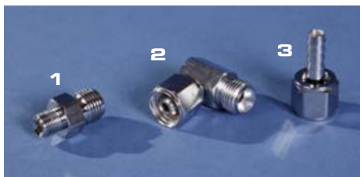
1) DISS 1240-AB Male Oxygen DISS 1/8" Male NPT 2) DISS 1240-ABE Female x Male Oxygen DISS Elbow 3) DISS 1240 Female Oxygen DISS 1/4" Tube Barb
