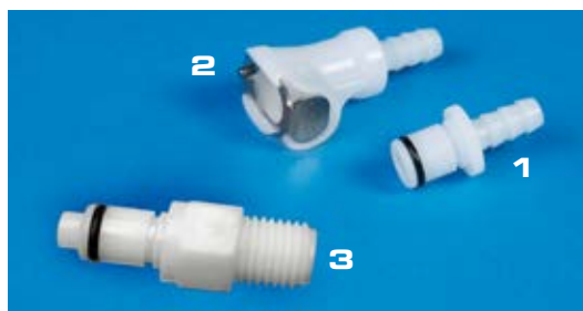
1) PLC-22004 1/4" Male plug to barb - straight through 2) PLC-17004 1/4" Female plug to barb - straight through 3) PLCD-240-04 1/4" NPT Male plug threaded - shutoff
