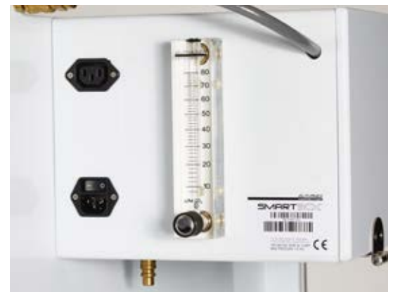
Integrated flow meter (80 LPM)
