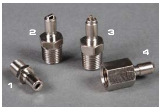
1) E-098 Male Quick Disconnect 1/8" Male NPT, 1-way valved 2) E-099 Male Quick Disconnect 1/4" Male NPT, 1-way valved 3) E-0992V Male Quick Disconnect 1/4" Male NPT, 2-way valved 4) E-099F Male Quick Disconnect 1/4" Female NPT, 1-way valved
