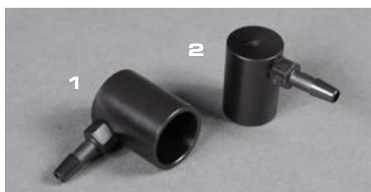
1) EZ-1501 Female 23mm Vaporizer Connector, Delrin Plastic 1/4" Tube Barb 2) EZ-1502 Male 23mm Vaporizer Connector, Delrin Plastic 1/4" Tube Barb
