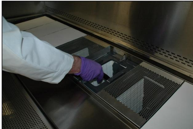
Direct the PAO from the generator outlet tube to the area of the HEPA prefilter that is exposed, Challenge the prefilters with the PAO wand by moving the generator outlet tube at a rate of 2cm per second and making sure the PAO is directed into the exposed pleats of the filter. Slow the traverse rate when a count of 50 particles every 2 seconds is detected, then re-scan the area of increased particulate release.
