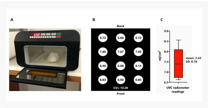
Figure 1. The UVP Crosslinker CL-3000 is a compact, high-intensity, high-uniformity irradiation device. A) Image of the CL-3000 with the front door open and N95 mask placed on the floor of the instrument. B) Diagram depicting the position and intensity of radiometer readings (units mJ/cm<sup>2</sup>). C) Box whisker summary plot of data from Figure 1B.
