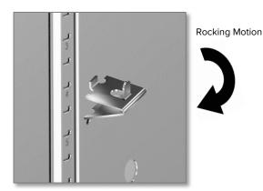
Figure 4: Installing Shelf Clip
