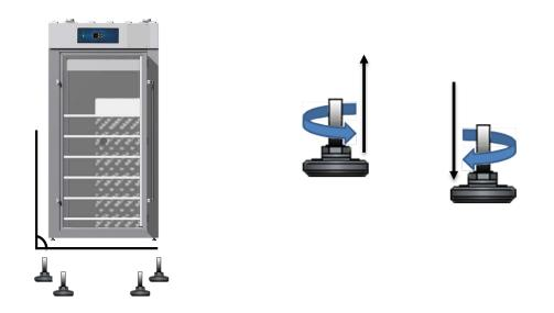
**Note:** To prevent damage when moving the unit, turn all 4 leveling feet so that the leg of each foot sits inside the unit.
