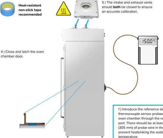
3) Place the sensor probes in the oven with the probe heads at least 2 inches (50 mm) from the surface of the shelving or walls to prevent heatsinking. Secure with non-stick, heat-resistant tape.
