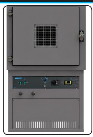
The SHEL LAB Model SVAC9-2 includes a Watlow temperature controller that can be programmed to perform multiple ramp and soak profiles. A digital vacuum gauge shows chamber vacuum level in measurements of Torr and m/ Torr. The display range is 760 Torr down to 0 mil Torr. A secondary independent high limit controller provides overtemperature safety protection.
