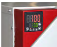
Controller with 7-segment display
