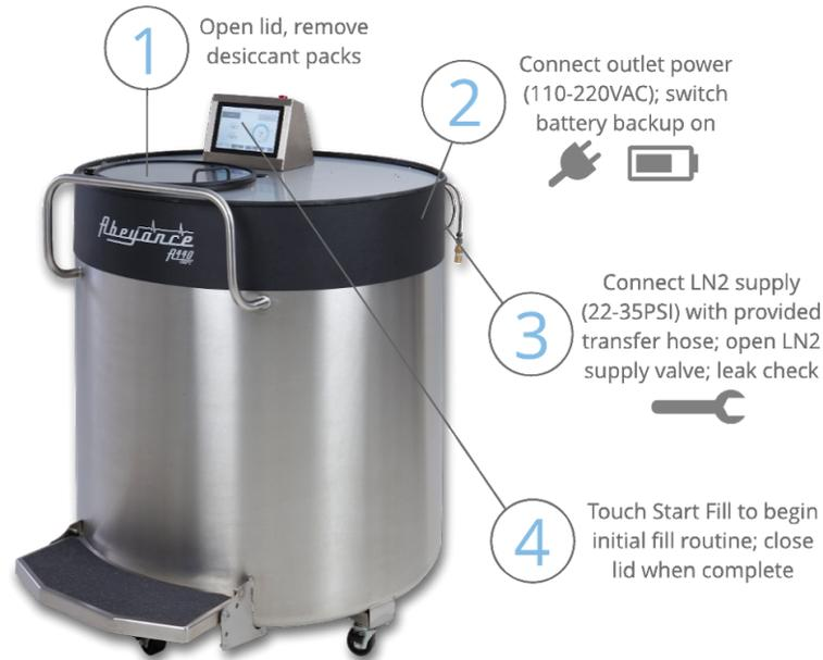
The initial fill can take 1-2 hours. When complete, normal controller operation will maintain LN2 levels while monitoring and logging storage conditions. Allow the freezer to cool for 48 hours before introducing samples. Routinely verify freezer status and ensure sufficient LN2 supply.
