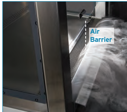
A dynamic air barrier at the front of the cabinet separates the laboratory from the work zone environment at an air speed of 105 fpm (0.53 m/s).
