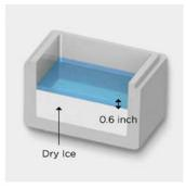
A dry ice-filled Styrofoam box is currently the standard method used for receiving, handling and transporting valuable frozen samples. However, only a 0.6 inch (1.5 cm) high zone above the dry ice stays below -50°C for 2 hours. Worse, at 2 inches (5.0 cm) above the dry ice - the top of a standard 2-inch cryostorage box- the temperature is above -20°C.
