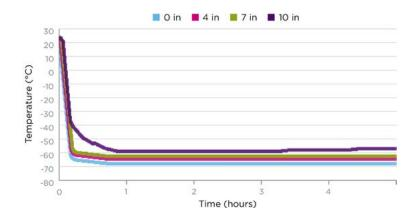
BioT™ ULT Workstation equilibrates to <-50°C in less than 30 minutes and entire chamber maintains temperature stability for over 15 hours. Temperature measured at 0 inches (blue), 4 inches (red), 7 inches (green), 10 inches (lavender).
