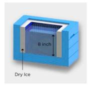
BioT™ ULT Transporter provides a stable ultra-low temperature (< -70°C to -50°C) work zone 8.0 inches (20.3 cm) deep. Up to 8 standard 2-inch cryostorage boxes will remain safely below -50°C for over 8 hours with the lid open and over 24 hours with the lid closed with one charge of dry ice.
