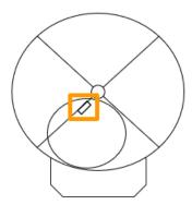
Figure 6-1: Measuring channel for manual LN<sub>2</sub> level confirmation located along freezer divider.
