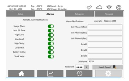
Figure 6-5: Alarm Notifications: local audio/visual, remote text and email, dry alarm contacts
