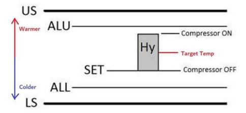
During the normal operation, the refrigerators (or freezers) compressor would turn on and off, to maintain the cold temperature in the storage chamber.
