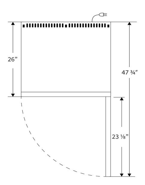
Note: This unit must have 4" clearance on sides and back for adequate ventilation
