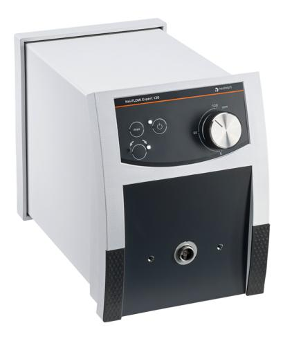
The pump drive of the model 120 of the Hei-FLOW Expert series can be operated with either single-channel or multi-channel pump heads. The flow rates with single-channel pump heads are in the range of 0.38 - 813 ml/min; with multi-channel pump heads from 0.005 - 329 ml/min.
