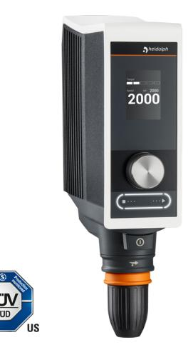
With Hei-TORQUE Expert 200 you can optimally stir viscosities up to 100,000 mPas or volumes up to 50 liters ( $H_2O$ ). Thanks to a wide speed range from 10 to 2,000 rpm and a maximum torque of 200 Ncm, it works particularly powerful.
